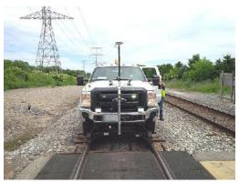
Figure 2. Hi-Rail Vehicle with RTK GPS.
