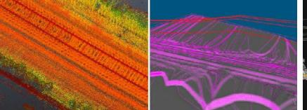
Figure 5. Classified pointcloud data shown by elevation (left). Surface mesh DEM-TIN (right).
